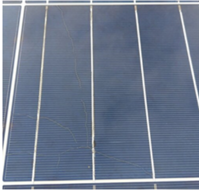
Figure 02 : Minor micro cracks in a solar cell
